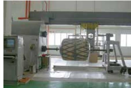
Waterco's Micron Commercial Fibreglass Filters are made from continuous strands of high quality fibreglass filament wound under controlled tension to create a seamless, impervious vessel. This produces a filter that is free from welds or seams, or special tank linings that typically corrode or electrolyse.
