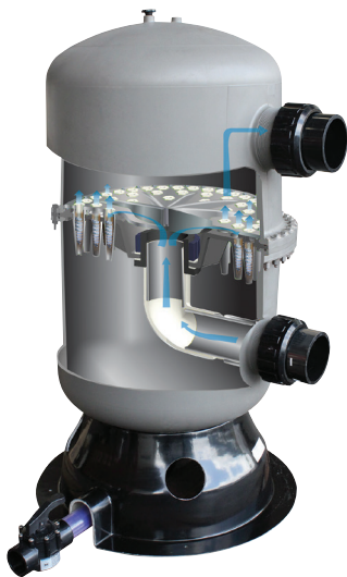
The MultiCyclone 70XL works on the basis of centrifugal water filtration, and there are no moving parts to wear and tear, and no filter media to clean or replace.
