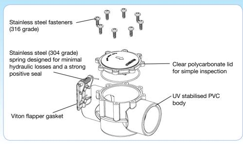
The Flow Check valve's pressure rating of 400 kPa (58 psi) and its 316 stainless steel fasteners make it suitable for domestic and commercial applications.
